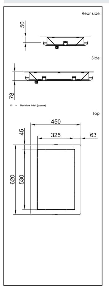
Drop-In Drop-in tempered glass top (1 GN container capacity)
