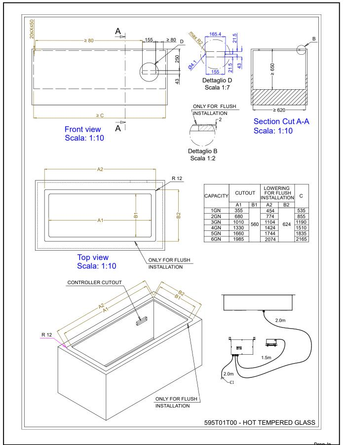
Drop-in tempered glass top (1 GN container capacity)
